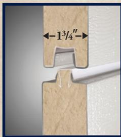
A **Full Thermal Break** is used in the tongue-and-groove construction of all 700 series doors. This rigid vinyl extrusion seals the joints and eliminates metal-to-metal contact, which limits the transfer of temperature.
