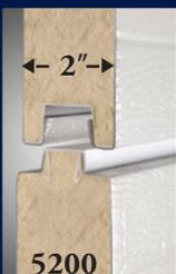
A Full Thermal Break is used in the tongue-and-groove construction of all 5000 series doors. This rigid vinyl extrusion seals the joints and eliminates metal-to-metal contact, which limits the transfer of temperature.
