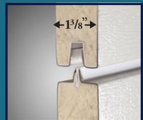
A **Full Thermal Break** is used in the tongue-and-groove construction of all 600 series doors. This rigid vinyl extrusion seals the joints and eliminates metal-to-metal contact, which limits the transfer of temperature
