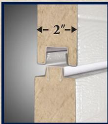
A **Full Thermal Break** is used in the tongue-and-groove construction of all 2000 series doors. This rigid vinyl extrusion seals the joints and eliminates metal-to-metal contact, which limits the transfer of temperature.
